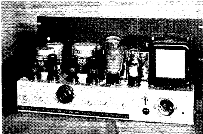
◆ Fig. 3 — Chassis view of the scanning unit. ◆
